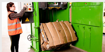
High compaction ratio creates the optimum 250 kg bale
